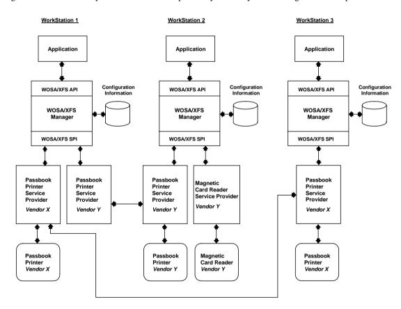
Figure 2 - An XFS architecture example for a branch office banking system.
